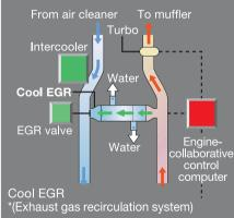
The **HINO 300** series is equipped with the latest EURO 4 compliant N-series engine which delivers excellent environmental performance with abundant power. The engine incorporates the cool EGR system as well as HINO's unique DPR (Diesel Particulate active Reduction system) to improve its environmental performance to meet the needs of the new age. In addition to being fuel efficient and quiet, the engine also delivers a resilience that allows it to be driven smoothly around the town.
